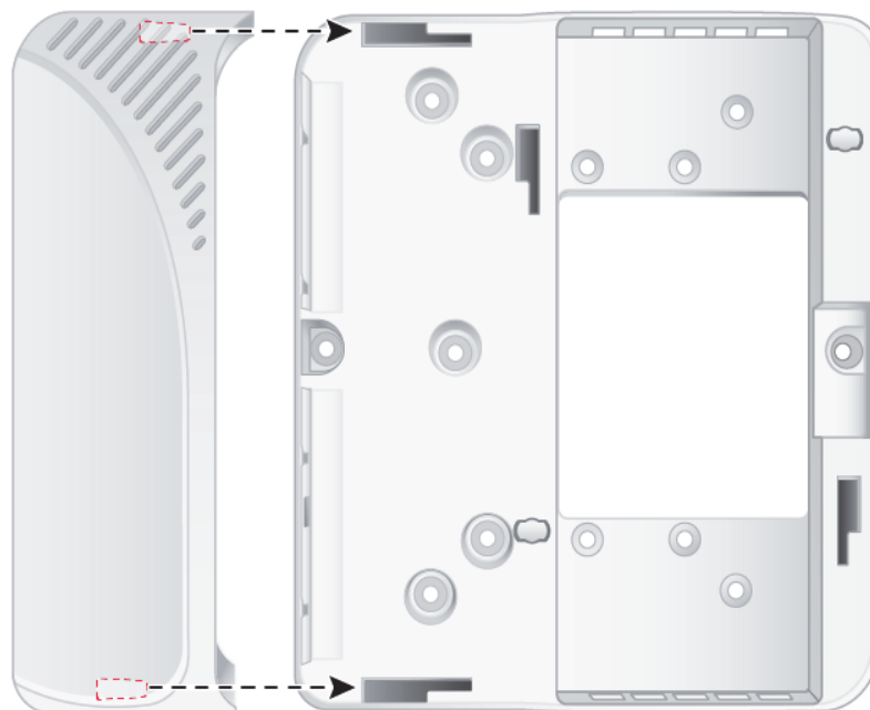
Figure 5 Fitting Front Cover onto Wall Mount
